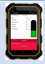
Converts cylinder liquid contents into weight. Streamex, SR200 & Inertec.
